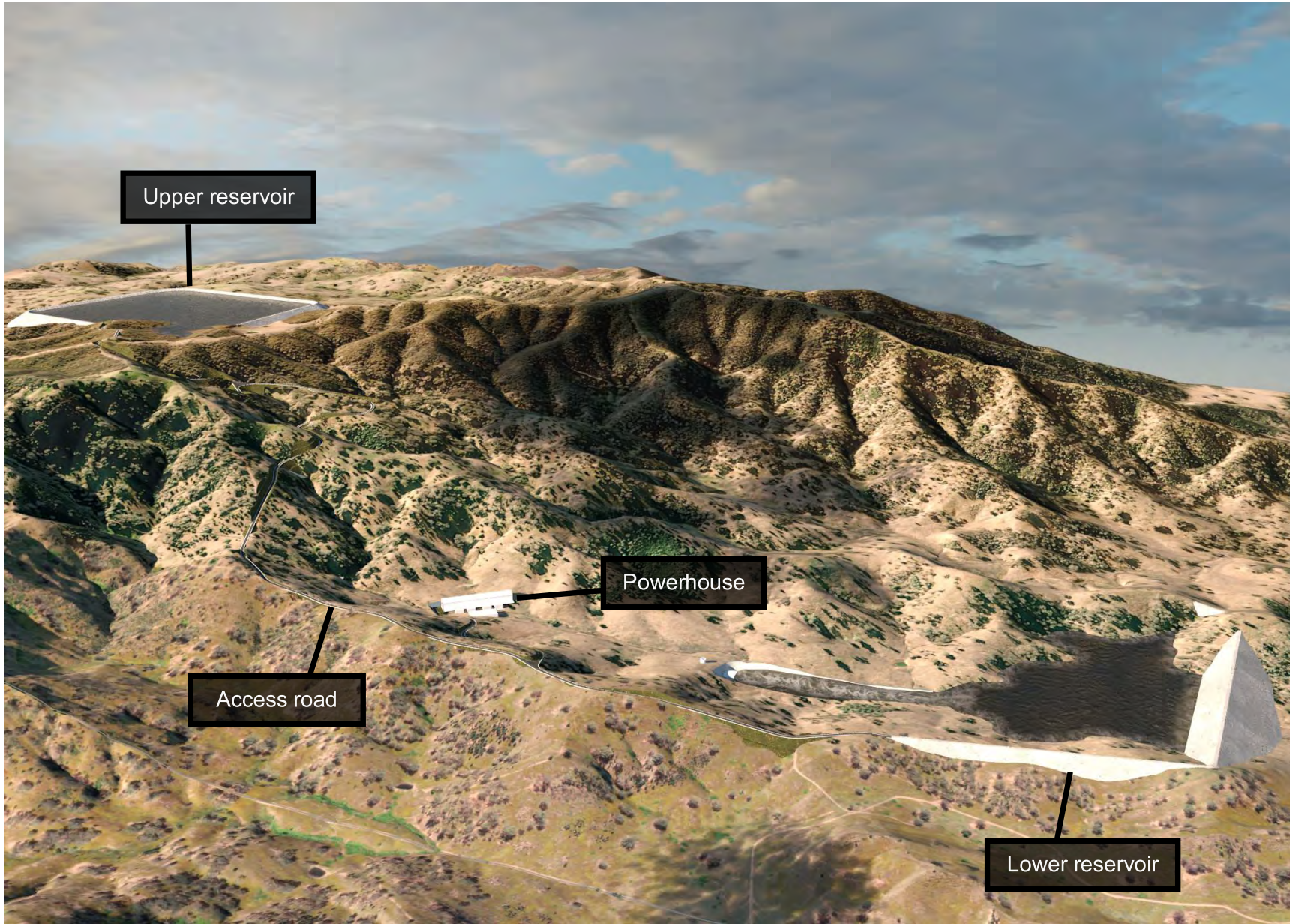
Figure 3.3 Upper and lower reservoir concept design
