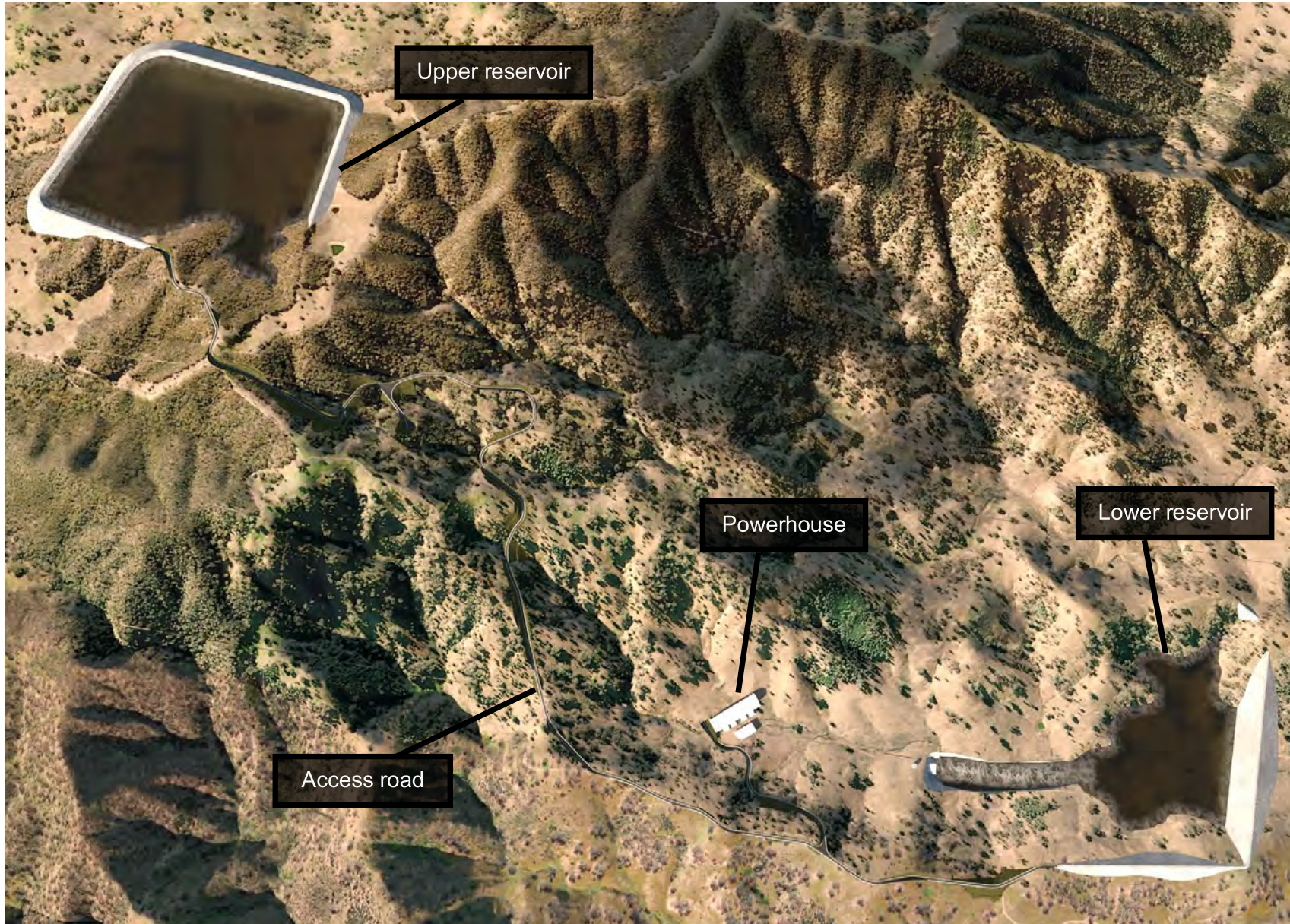
Figure 3.2 Upper and lower reservoir concept design
